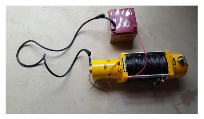
For winches with the larger 8.9hp motor, the black earth cable connection is underneath the motor.
