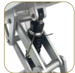
Shock absorber pressure adjustment knob with supplied allen keys
